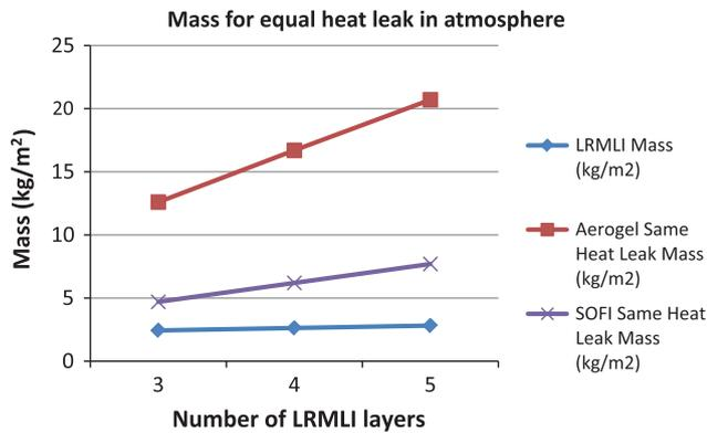
Fig. 5. Insulation mass required for equal heat leak to 3, 4 and 5-layer LRMLI.
