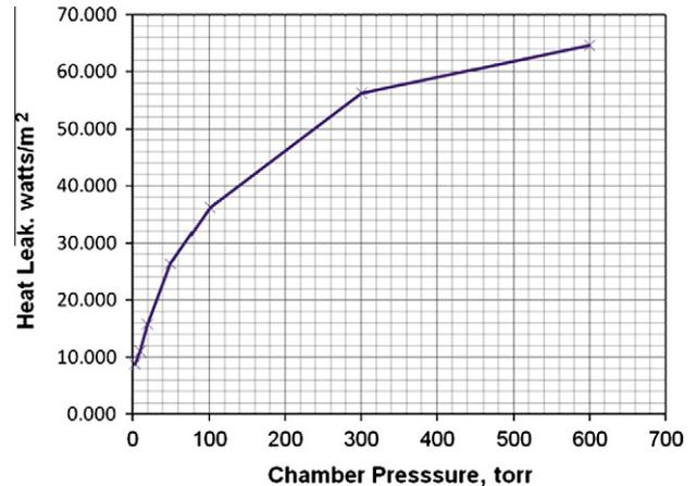
Fig. 3. LRMLI heat leak from 295 °K to 77 °K as a function of external atmospheric pressures.
