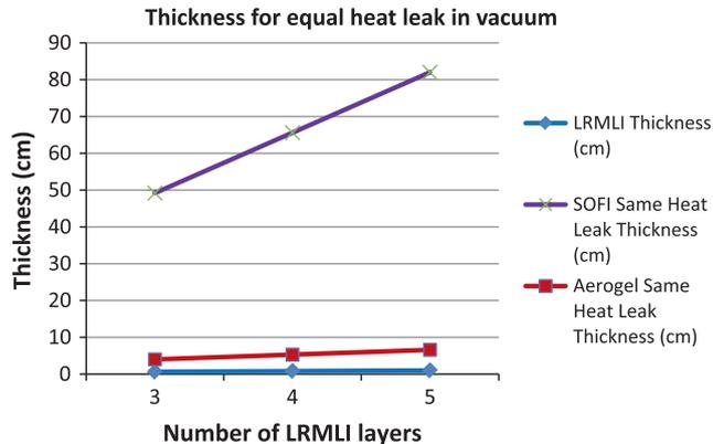
**Fig. 6.** Insulation thickness required for equal heat leak to 3, 4 and 5-layer LRMLI.
