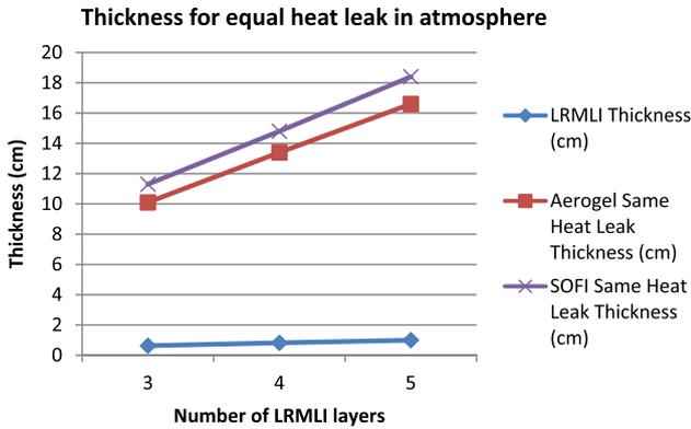
Fig. 4. Insulation thickness required for equal heat leak to 3, 4 and 5-layer LRMLI.
