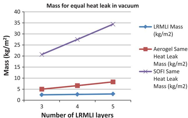
**Fig. 7.** Insulation mass required for equal heat leak to 3, 4 and 5-layer LRMLI.
