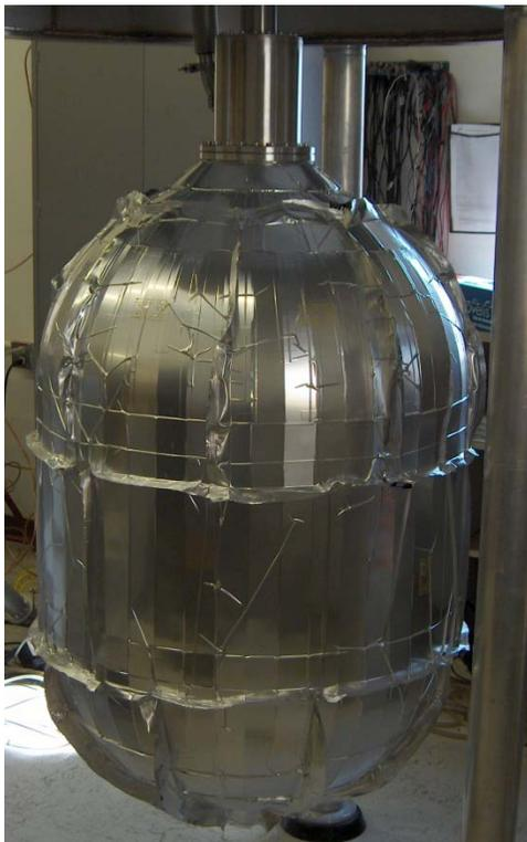
The 400 liter tank was a cylinder 30 inches in diameter with hemispherical heads and was 45 inches long. A photo of the LRMLI installation, under vacuum, on the 400 liter tank is shown in Figure 2.
