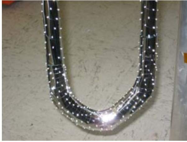
FIGURE 5. WMLI prototype layer 4 installed around bends in tubing.
