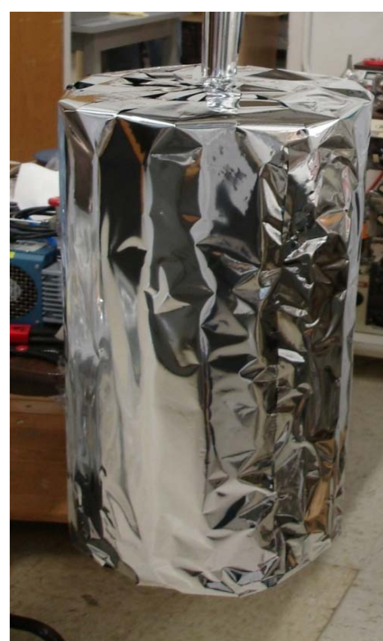
Cylindrical LN 2 tank insulated with cylindrical IMLI blanket.
