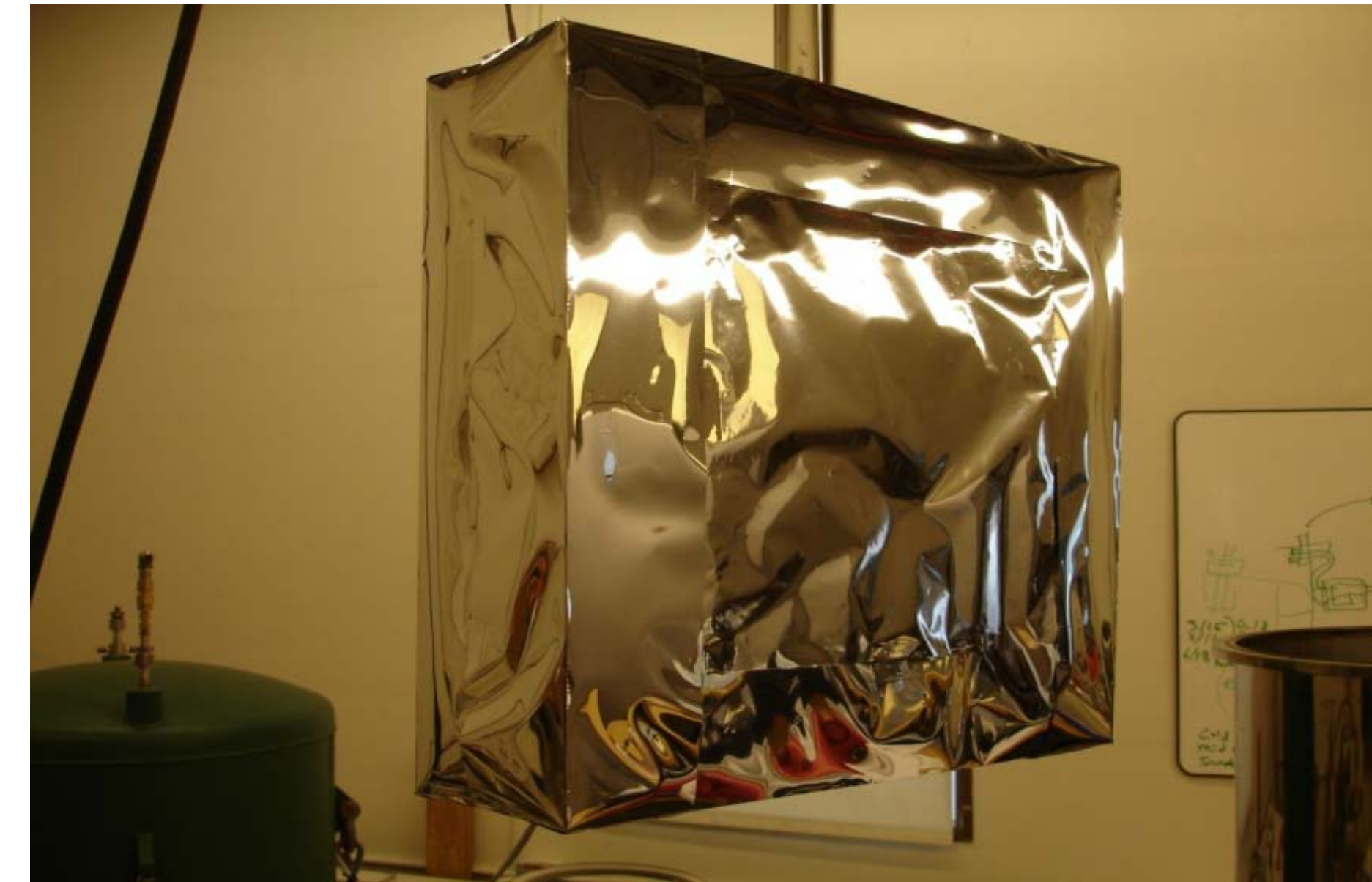
Rectangular LN 2 tank insulated with IMLI blanket, used for boil-off calorimetry to measure thermal conductance of IMLI.
